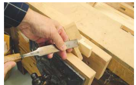
▲ Pic.21 The outer faces will need the mouldings mitred at the top corners and cut out to sit on the sill
